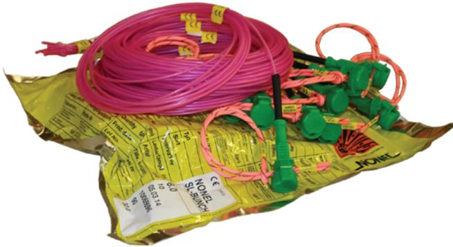
NONEL<sup>®</sup> Bunch Connectors are quick-connection units that can initiate 5 to 20 NONEL tubes at the same time. The standard NONEL Bunch Connector consists of a SLO connector block (green) that contains a mini-detonator with no delay element. A loop of detonating cord, dimensioned to initiate a bunch of NONEL tubes, is connected to the SLO connector block. Several bunches of NONEL tubes can be initiated at the same time.
